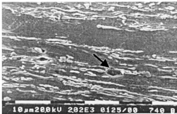
Figure 6 Microvoid formation near the fracture surface for 740B18.
